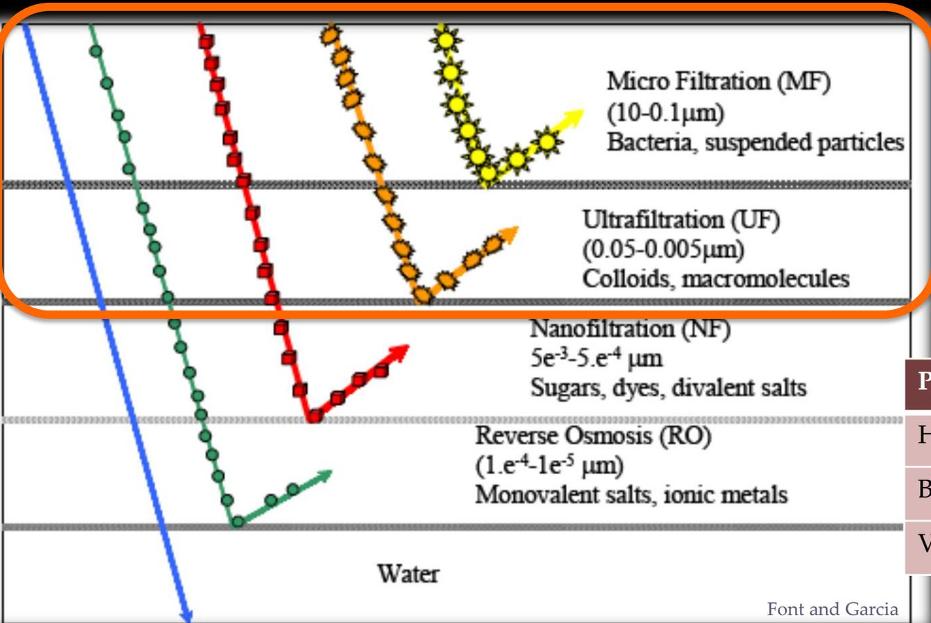
Membranes provide an absolute physical barrier for pathogen removal for safe dewatering
