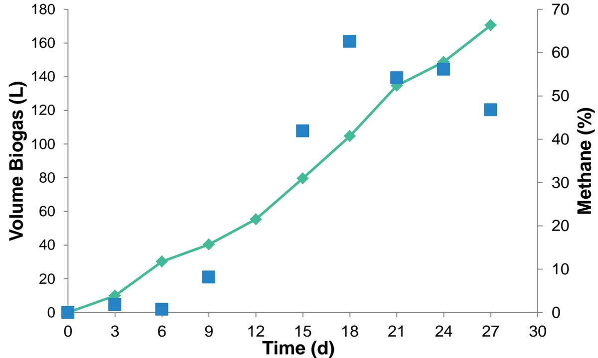
◆ Cumulative Volume of Biogas    ■ % Methane
